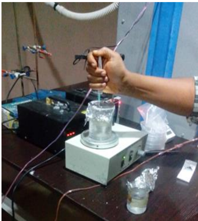
Plate 1: Addition of sodium hydroxide solution to that of zinc acetate
